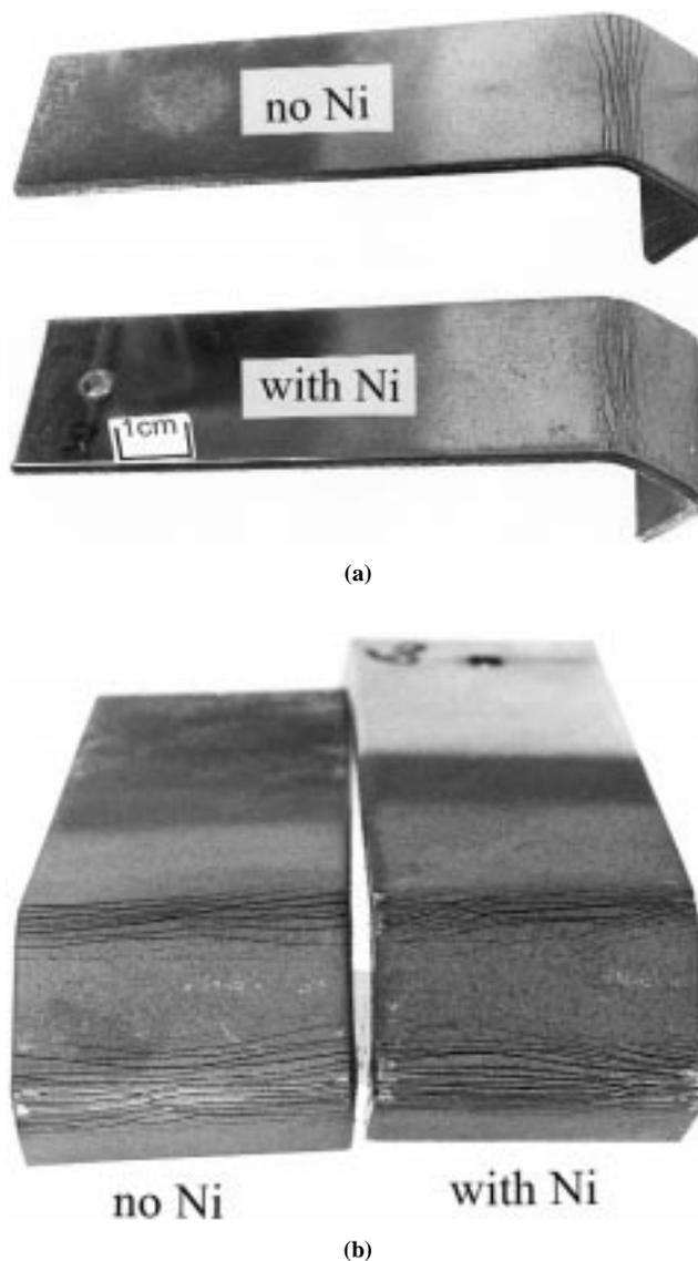
**Fig. 1** Specimens after bending test. (a) Specimen size and bending angle. (b) Details of bent surfaces
