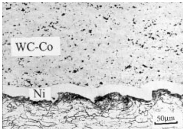
**Fig. 3** The microstructure of specimen 1
